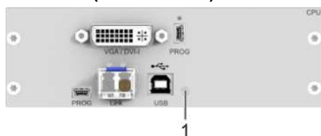
Fig. 54 Interface side extender module - Failure indication L474-BShxV
