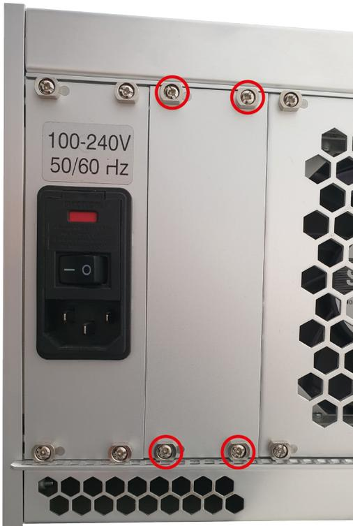
Fig. 81 Removing the blanking plate from chassis 474-BODY21/4U
